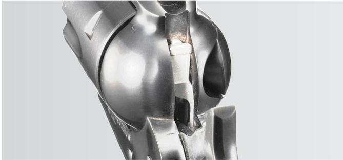
The transfer bar and loading gate interlock provide an unparalleled measure of security against accidental discharge if the user fails to take basic safety precaution of keeping the hammer down, over an empty chamber.
