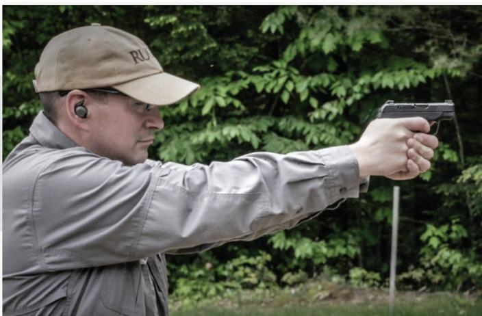
Function testing involves firing a specified amount of ammunition to ensure the firearm will operate reliably and without malfunction, out of the box.
