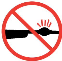
Before loading or shooting the **SFAR™**, be certain the bore is unobstructed. Firing the rifle with any obstruction in the bore may result in severe damage to the rifle and serious injury to the shooter and other persons nearby.
