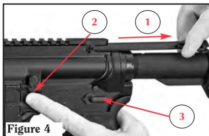
**To release the bolt carrier** (which allows the bolt to move forward) keep selector on "SAFE" and either:
