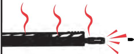
The SFAR™ fires from a closed bolt. Sustained firing can create excessive heat in the barrel and can cause “cook-off” of ammunition (heat-firing of the cartridge in the chamber). This “cook-off” can occur a substantial period of time after firing has ceased. Always unload the firearm and unload the chamber immediately after you have finished shooting.
