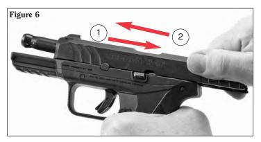
5. Retract the slide appoximately 1/16" so the front of the slide aligns with the front of the grip frame. Pry loose the takedown pin using a non-marring armorer's tool or other flat, blunt tool (see Figure 7).
