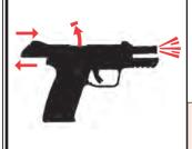
The slide automatically opens and shuts quickly while firing. Keep face and hands away from rear. Hot brass is ejected quickly and can burn you. Always wear shooting glasses and hearing protection.
