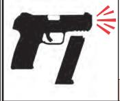
So that the pistol can be used as a single loader, it will fire whether or not a magazine is in the firearm if a cartridge is chambered. Removing the magazine does not unload pistol! To unload, <u>first</u> remove magazine, <u>then</u> pull slide to rear, eject chambered cartridge, and <u>visually inspect chamber</u> to be sure it is empty. Always point the pistol in a safe direction when loading or unloading.
